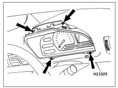
9.4a Instrument cluster securing screws (arrowed)
